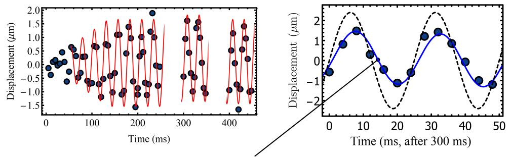
Fit steady-state response to  $R_{\alpha}(t) = A_{\alpha} \cos \left[\omega t - \phi_{\alpha}\right]$
