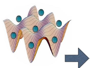
Atoms: counterpropagating laser beams produce a sinusoidal potential
